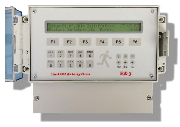
EZ3 is a central monitoring and control equipment for up to 999 EmLOC end devices.
